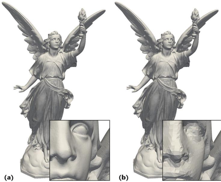
Figure 8. Example of mesh simplification. (a) Original mesh and (b) a mesh simplified on a  $512^3$  grid of bins.
