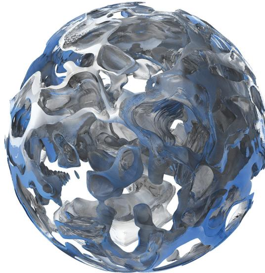
Figure 2. Example output from VTK-m ray-tracing algorithm. The data in this rendering represent seismic wave propagation through the Earth.
