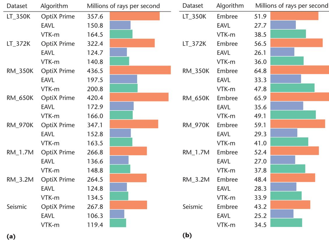
Figure 3. The speed (measured in millions of rays cast per second) to perform ray tracing using different algorithms on different data sets. (a) GPU times and (b) CPU times. The datasets are the same ones used in the Larsen study,<sup>10</sup> as are the timings for the Optix Prime, Embree, and EAVL algorithms.
