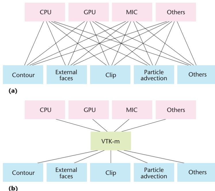
**Figure 1. VTK-m’s abstract device model. (a) Implementing all of our visualization algorithms separately for every architecture we need to support leads to an unmanageable amount of software. (b) By using VTK-m’s abstract device model based on data parallel primitives, we can reduce the amount of software to implement to a feasible level.**
