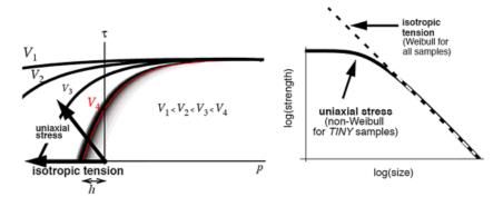
Fig. 2. The Weibull scale effect is applied only on the pressure intercept. The curved lines on the left plot are median limit surfaces for different specimen volumes showing that, as shown in the plot on the right, strength remains bounded for any stress path, such as uniaxial stress, having a deviatoric component.
