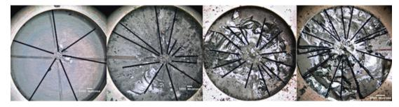
Fig. 10. Increase in radial cracking in boron carbide experiments due to an increase in impact velocity from 100 m/s (left) to 400 m/s (right).
