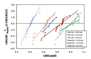
Fig. 4. Brazilian Weibull distribution and volume scaling of silicon carbide.
