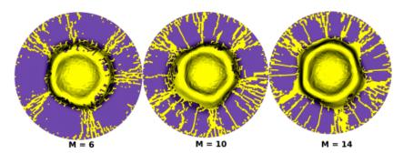
Fig. 11. Weibull modulus effect on radial cracking in boron carbide simulations impacted at 400 m/s.
