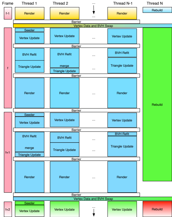
Figure 2: Given a highly parallel architecture with N parallel threads, we spend N-1 cores on parallel rendering and BVH refitting. The N 'th thread works asynchronously and builds new BVHs as fast as possible, potentially over multiple frames (2 in this example); in the meantime, the render threads rely on deforming the most recently finished BVH. BVHs are never deformed for more than a couple of frames, and both scalability bottlenecks and pauses are avoided altogether.
