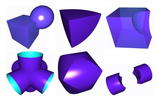
**Figure 2** Toy examples. *First row*: union, intersection and difference of a cube and a sphere (20, 160, and 28 fps). *Second row*: union, intersection and difference of three cylinders (91, 84, 127 fps).
