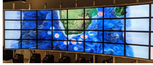
Figure 6: Unstructured volume raycasting in our prototype GPU renderer run locally on six nodes, each with two GTX 1070s.
