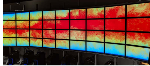
Figure 7: Data-parallel rendering of the 500GB DNS volume (10240×7680×1536 grid) with OSPRay on 64 SKX nodes on Stampede2, streamed to the POWERwall in direct mode, averaging 6-10 FPS.
