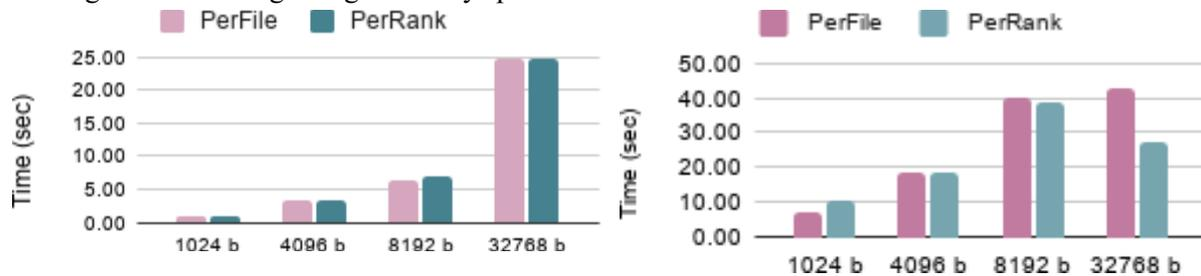
**Figure 2.** Time (in seconds) needed to complete some read operations on a single core on Summit versus the number of blocks in a single ADIOS variable. We see that the time needed generally increases as the number of blocks increases.
