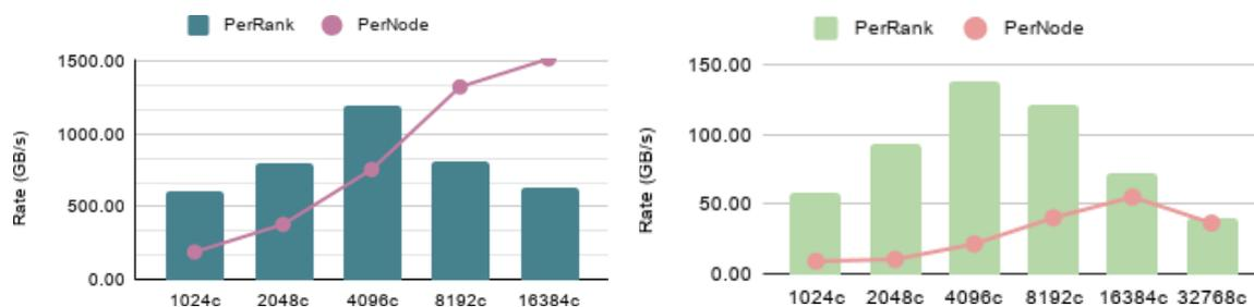
**Figure 1.** Weak-scaling performance of two ADIOS writing options, one subfile per MPI rank and one subfile per compute node. These options reduce the dependencies among the compute nodes and are typically the most performant options.
