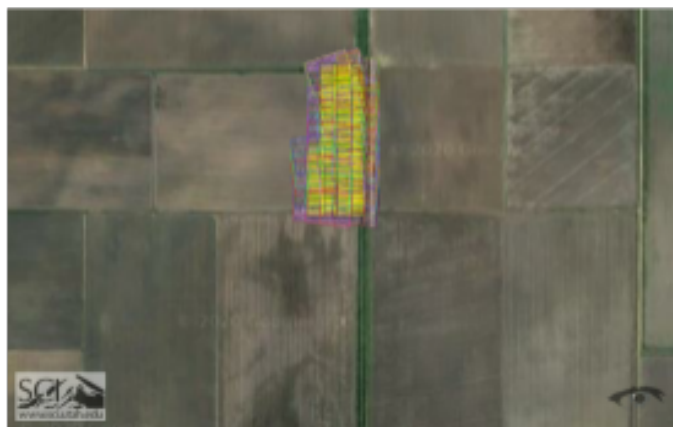
Figure 2. The ViSUS ViSOAR Ag Explorer has demonstrated that actionable information can be obtained directly on the field thanks to its fast stitching and data streaming technology, as shown with this example of a georeferenced mosaic of aerial images registered on Google Maps.
