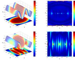
**Fig. 1.** (*left*) Functions displayed on corrugated surface mesh and its projection onto the x-y plane and (*right*) relative error of gradient approximations at simulated corrugated surface mesh nodes projected onto the x-y plane. Results for (*top*) cylindrical and (*bottom*) ellipsoidal radial logistic functions.
