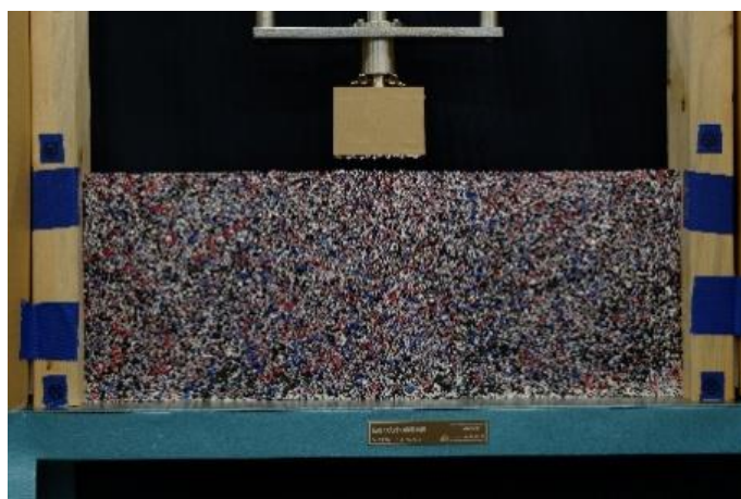
Figure 6 : Arrangement of shallow foundation loading test equipment
