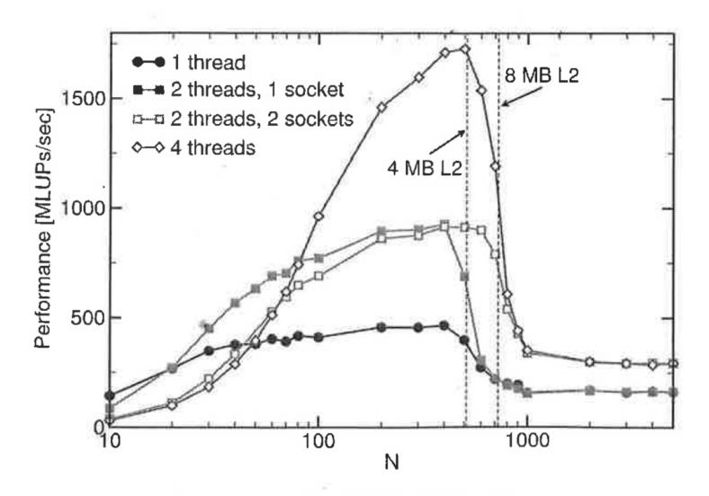
Performance of an OpenMP Jacobi Code on an Intel Dual Core Dual Socket Xeon 5160 3Ghz. For two threads there are 2 choices wrt how the sockets are used Breakdown in perf. with increasing N when memory does not fit into cache any more.
