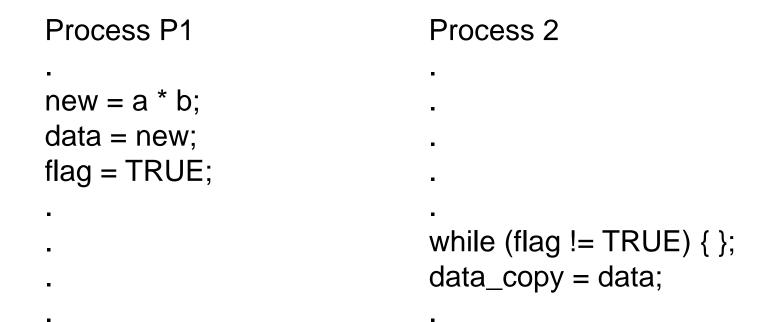
Multiply machine instruction corresponding to new = a \* b is issued for execution. The next instruction corresponding to data = new cannot be issued until the multiply has produced its result. However the next statement, flag = TRUE, is completely independent and a clever processor could start this operation before the multiply has completed leading to the sequence:
