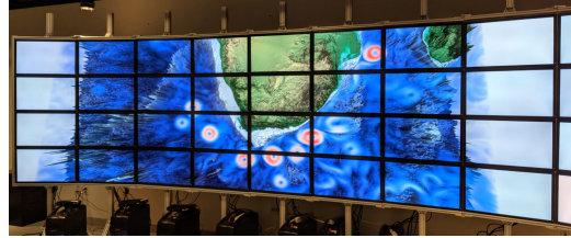
Figure 6: Unstructured volume raycasting in our prototype GPU renderer run locally on six nodes, each with two GTX 1070s.
