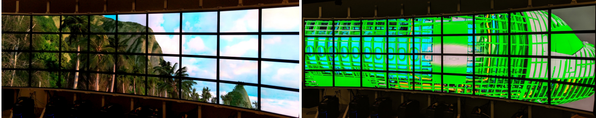
Figure 1: Left: The Disney Moana Island [18] rendered remotely with OSPRay’s path tracer at full detail using 128 Skylake Xeon (SKX) nodes on Stampede2 and streamed to the 132Mpixel POWERwall display wall, averages 0.2-1.2 FPS. Right: The Boeing 777 model, consisting of 349M triangles, rendered remotely with OSPRay’s scivis renderer using 64 Intel Xeon Phi Knight’s Landing nodes on Stampede2 and streamed to the POWERwall , averages 6-7 FPS.
