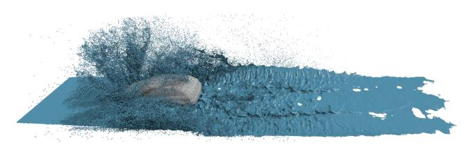
**Figure 1:** Watercrossing simulation using 2.1 million particles. Rendered at 4K resolution with ambient occlusion and hard shadows in 2.4 seconds on 32 Xeon Phi KNL nodes of the Stampede2 supercomputer.
