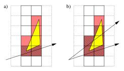
Figure 5: While one ray (a) can re-visit a triangle in multiple cells only along one dimension, a frustum (b) visits the same triangle much more often (even worse in 3D). These redundant intersection tests would be costly, but can easily be avoided by mailboxing.
