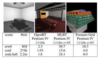
Table 2: Static scene ray tracing performance for both the packetized grid, OpenRT, and MLRT. OpenRT and MLRT data are taken from [Reshetov et al. 2005]; all times are including simple shading, but without display. Though these three scenes are best-case examples for our competitors, we remain at least competitive.
