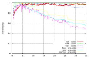
Figure 6: For several different models, this graph shows the framerate, normalized by the best time, in relation to grid size as determined by  $\lambda$  (on the X axis). Nearly all tested scenes, both static and dynamic, reach their optimum at approximately  $\lambda \approx 5$ .
