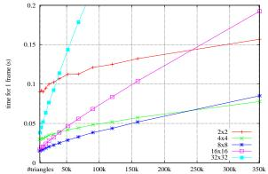
Figure 7: Static render time with varying packet sizes and different resolutions of the Stanford Armadillo. There is a crossover point around 250K triangles where  $4 \times 4$  packets become more efficient than  $8 \times 8$  packets. Nevertheless, both  $4 \times 4$  and  $8 \times 8$  show nearly the same performance over a wide range of model complexity.
