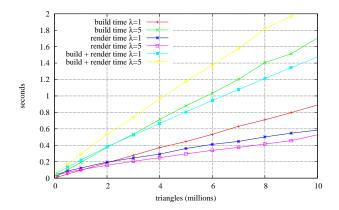
Figure 8: Rebuild and render times at  $\lambda = 1$  and  $\lambda = 5$  for different resolutions of the Stanford Thai Statue ranging from 100K to 10M triangles. For these large models, we use a packet size of  $4 \times 4$ .
