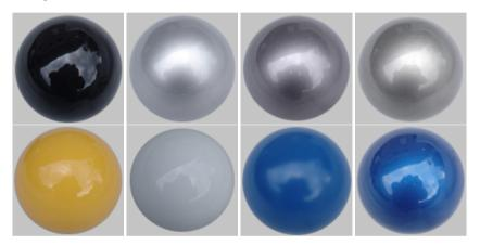
Figure 9: Our sphere-samples painted with different car paints. Top row: Metallic car paints. From left to right: Ford F8, Polaris Silber, Opel Titan, and BMW 339. Bottom row: Standard car paints. From left to right: 2K Acrylack, White, Blue Matte, and Blue.
