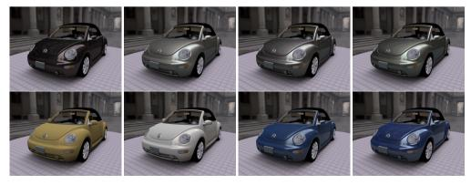
Figure 10: Rendering results with different measured and fitted car paints. From left to right, top to bottom: Ford F8, Polaris Silber, Opel Titan, BMW 339, 2K Acrylack, White, Blue Matte, and Blue.
