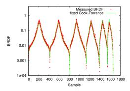
Figure 5: Fitting example of measured "Polaris Silber" BRDF data with a two-lobe Cook-Torrance model.
