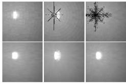
Figure 4: Comparison of different BRDF parameterizations. Top Row: Without interpolation and hole-filling, empty bins marked with black. Bottom Row: With interpolation and hole-filling. Left: Traditional BRDF parameterization. Center: Linear halfway vector based parameterization. Right: Halfway vector based parameterization with nonlinear sampling of  $\theta_h$ .
