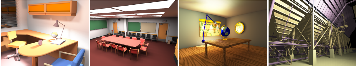
Figure 26: Instant Global Illumination. a.) Office scene, with soft shadows, reflections, refractions, and a caustic from the glass ball. b.) Conference scene with 280,000 triangles and 220 light sources, c.) Global Illumination in an animated VRML scene, and d.) Global Illumination in the 12.5 million triangle “power plant” scene. All scenes run interactively with several frames per second at 640x480 pixels while allowing interactive updates to the scene. Note that a.) was rendered with the older system, as caustics are currently not supported in the new version.
