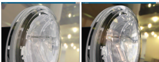
Figure 3: Enhanced visual quality using a High Dynamic Range Environment Map: Low dynamic range rgb environment map on the left, and a high dynamic range environment map on the right.
