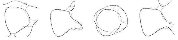
Figure 1: Classical least squares algorithm gives unstable 4^{th} degree IP fits under even the smallest perturbations to the data.
