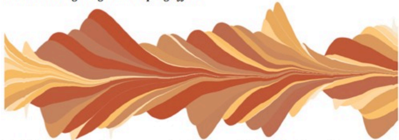
fig 14 – the same data set sorted using the weighted “inside out” strategy to highlight the initial onset of each time series
