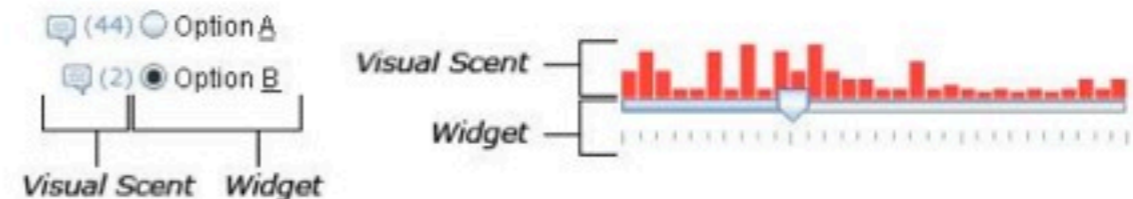
Figure 1. Widgets with visual information scent cues. Left: Radio buttons with comment counts. Right: Histogram slider with data totals.
