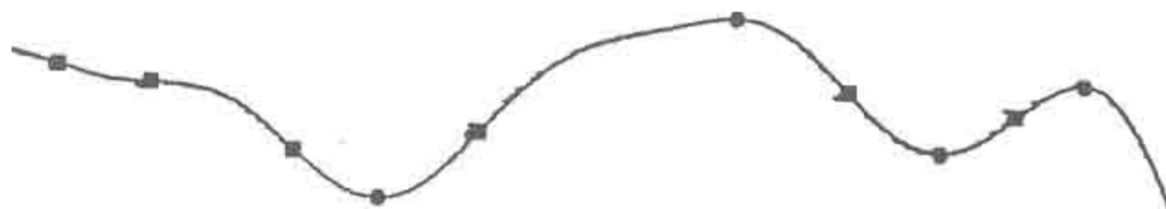
Figure 2 A function characterized by its extrema and those of its first derivative.
