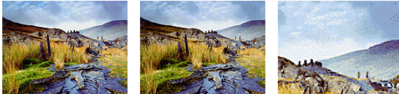
Figure 1.5 An example of color-dithering in image compression. Left: the original image, 26 KByte. Middle: color dithering, effective spreading of a smaller number of color pixels so that the blurring of our perception blends the colors to the same color as in the original. Filesize 16 Kbyte. Right: enlargement of a detail showing the dithering. From http://www.digital-foundry.com/gif/workshop/dithering.shtml .
