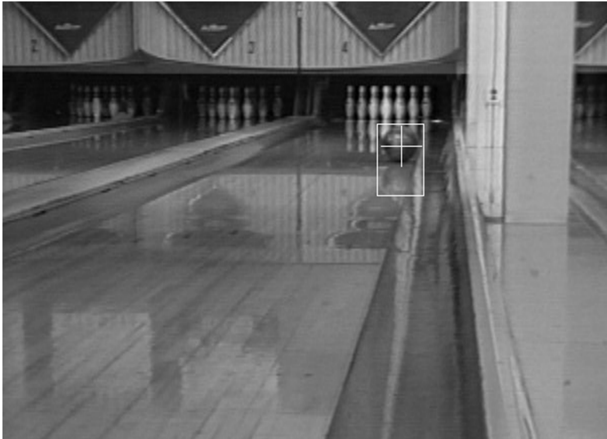
Crosshair indicates results of Hough transform, bounding box found via motion differencing.
