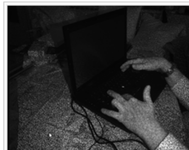
This infrared image shows the laser grid Kinect uses to calculate depth
