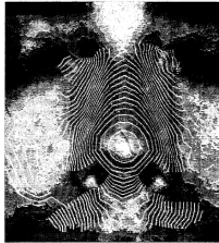
Figure 11-7. The shape-from-shading method is applied here to the recovery of the shape of a nose. The first picture shows the (crudely quantized) gray-level image available to the program. The second picture shows the base characteristics superimposed, while the third shows a contour map computed from the elevations found along the characteristic curves.
