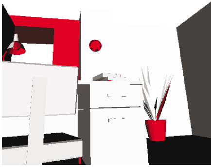
Fig. 2. Illustration of the accuracy of PLP: For the same viewpoint and model as shown in Fig. 1, the visible geometry that PLP rendered is shown in white and the visible geometry that PLP did not render is shown in red.
