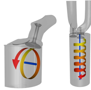
Fig. 11. Idealized in-cylinder flow through a gas engine (left) and a diesel engine (right). Figures 12 and 13 show our visualization of CFD data simulating such flows.
