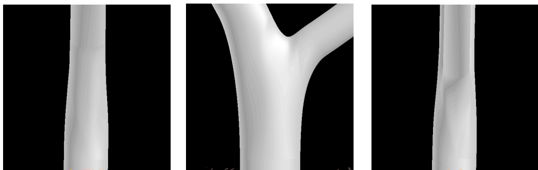
Figure 7.29. The bifurcation after 10,000 iterations to enforce tangent plane continuity along 6 of 21 boundaries.
