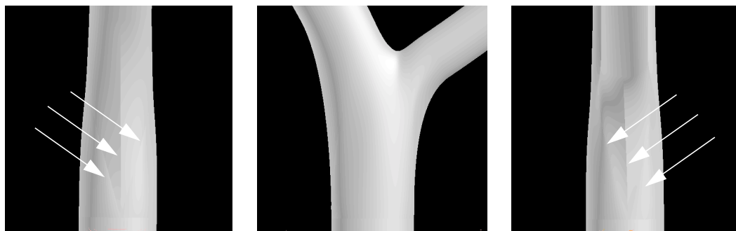
Figure 7.28. Initial bifurcation before the enforcement of tangent plane continuity. The arrows indicate the boundaries that are not tangent plane continuous.
