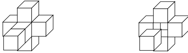
Figure 4.5. Incorrectly thinning of the central voxel from a 26 connected solid object using only the surface connectivity (object has been split into two parts).
