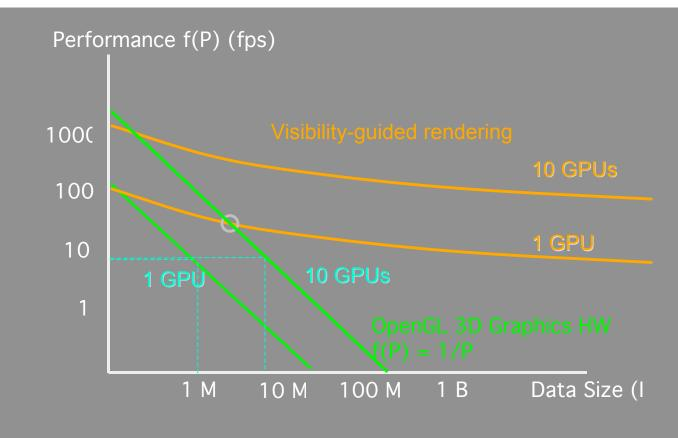
Already with one GPU, Visibility-Guided Rendering VGR is faster than direct hardware rendering witb 10 GPUs.
